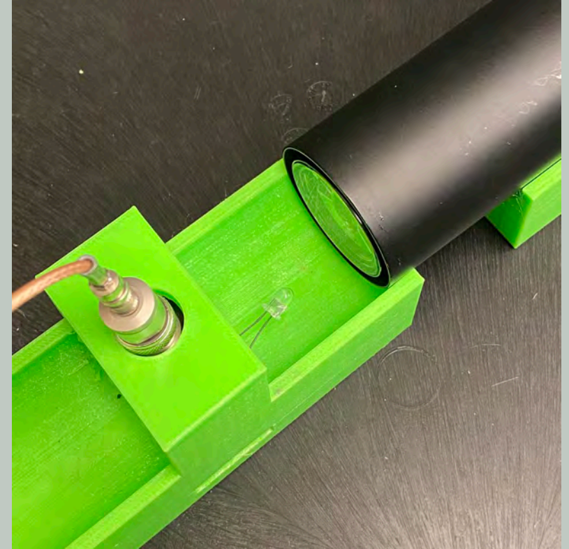
Figure 2. Concept design using an LED that pulses in sync with the reading of a photo-multiplier-tube.
